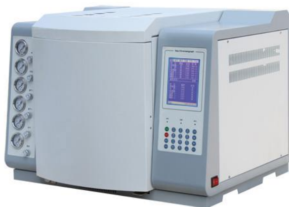
Fig.1.5 The appearance of HZGC-1212AIII gas chromatograph
